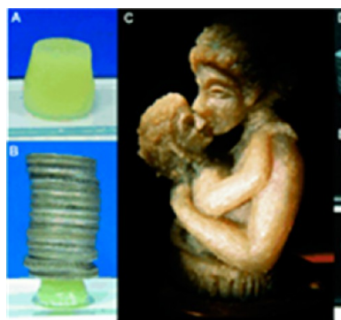
Figure 9. (A) 7.0 wt % GLY-C-in-nitrobenzene gel. (B) Gel from panel A under ca. 117 g of weight. (C) Gel from panel A carved into a sculpture of a mother holding a child. The author saw this sculpture in a hermetically sealed case (to avoid solvent loss) in Kolkata ca. 2 years after it was made; it was still in good condition. Reprinted with permission from ref 115. Copyright 2012 Wiley-VCH Verlag.
